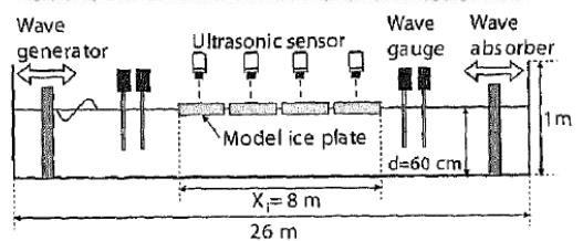
Fig. 3. The wave tank and experimental equipment.
