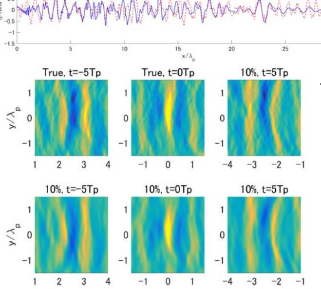
Example of a 2D reconstruction, mimicking assimilation of stereo image 2D wave field.
